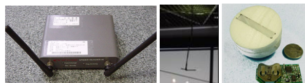
Figure 4: RFID reader, antenna attached to ceiling, and tag
