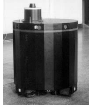
Fig. 2. 3-DOF omni-directional mobile robot
