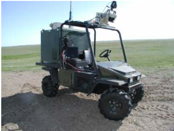
Fig. 2. Raptor Unmanned Ground Vehicle. Each Raptor used one or more roof mounted SICK lasers and stereo cameras; Differential GPS and IMU; and wireless mesh networking routers.
