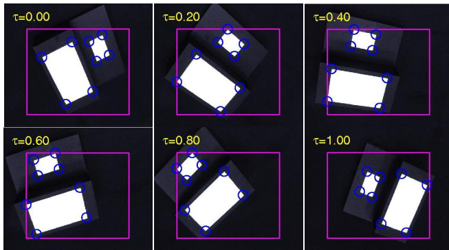
Fig. 9: Object identified during visual servoing along path planned with Algorithm C at instant \tau , seen by the camera.
