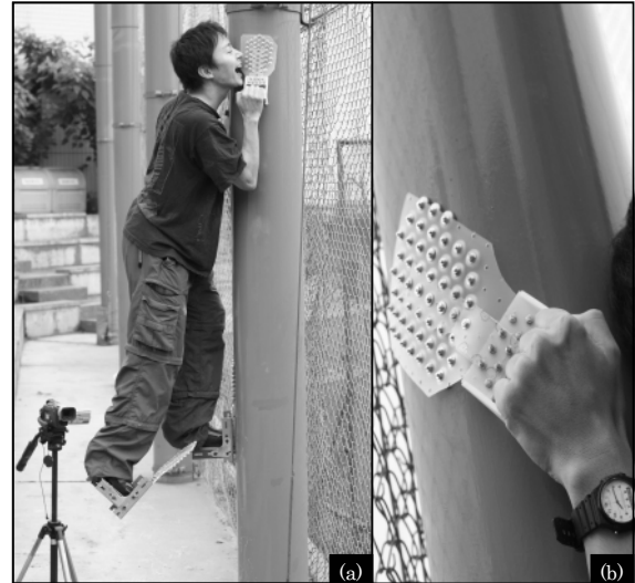
Fig. 9 Pole Climbing (a) A 58kg volunteer using Magnetic Pads to watch a game from a high vantage point. (b) Close-up. Adaptability to round surface: a pole.
