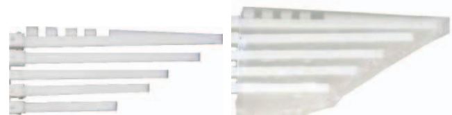
Fig. 13 Fin without and with flexible skin
