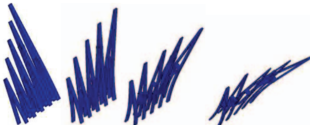
Fig. 11 Independently bending ribs forming pectoral fin curvature
