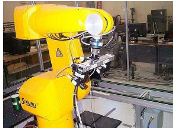
Fig 2. Staubli RX-130 robot carrying Biclops.
