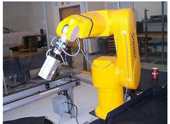
Fig 5. Staubli RX-130 robot carrying a laser pointer tool.
