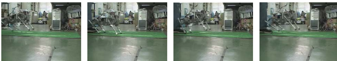
Fig. 6. Snapshots of Rush running in the bounding gait.
