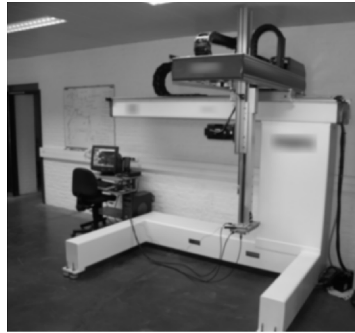
Fig. 3 Overview of the first test-setup prototype (stroke [mm]: X-1000 Y-400 Z-800, maximum feedrate: 120 m.min -1 , maximum acceleration: 4 m.s -2 ).
