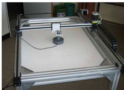
Fig. 6. X-Y plotter robot for the sensor investigation
