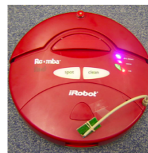
Fig. 1. The Roomba available off-the-shelf for US$150, along with its built-in sensory and actuation abilities. Proprioception is both capable and complete. Yet it has almost no sensing that reaches beyond the platform itself.
