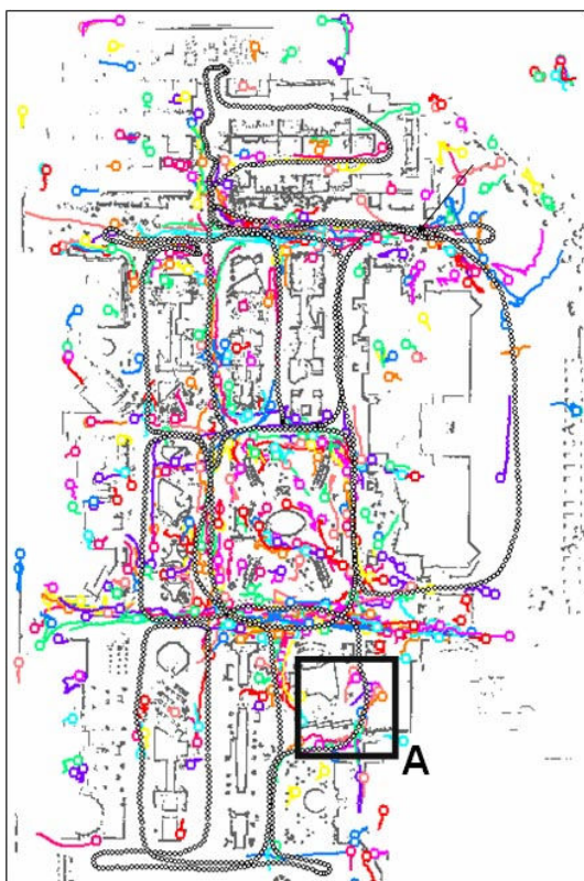
Fig. 9. Experimental results at the exhibition hall: background map, sensor's motion trajectory, and all detected pedestrian trajectories
