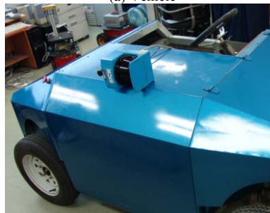
(b) The proposed sensor system attached to the vehicle Fig. 8. Vehicle for outdoor experiment
