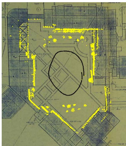
Fig. 12. Overlapping the result with the floor plan of the building (Yellow: reconstructed walls, Black: estimated motion)
