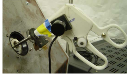
Fig.7 Joy-stick type manipulator for remote control
