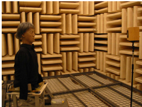
Fig. 3. Photograph of the experiment. Dummy head 3 (DH3) was set on TeleHead in an anechoic room. A loudspeaker was set 1.2 m in front of TeleHead .
