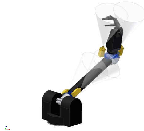
Fig. 2. Multiple vision sensor network on the robot arm
