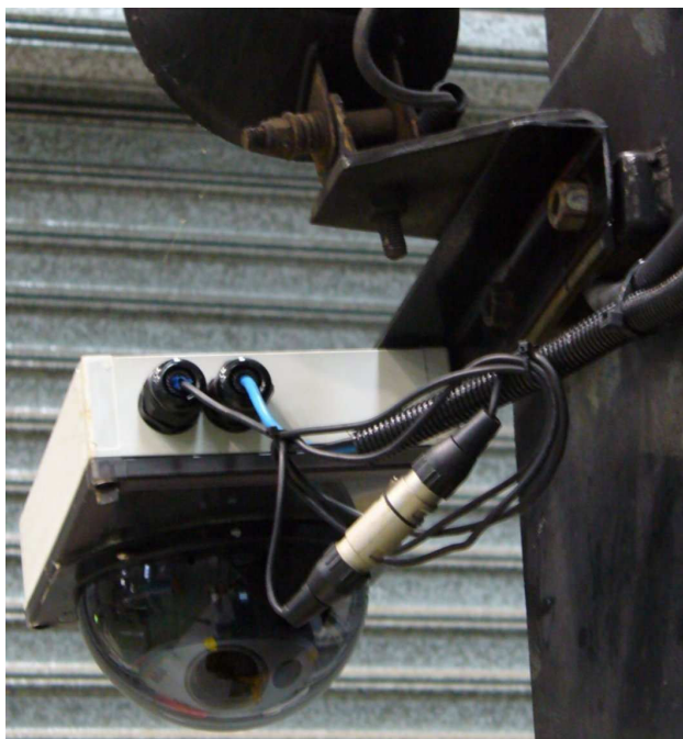
Fig. 3. The PTZ camera used for locating the crucible.
