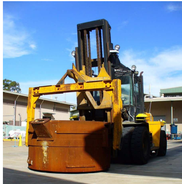
Fig. 1. A Hot Metal Carrier in the process of picking up the crucible.
