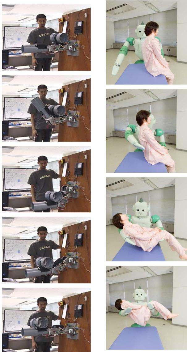
(a) Handling task using arm (b) Human care task using RI-MAN
