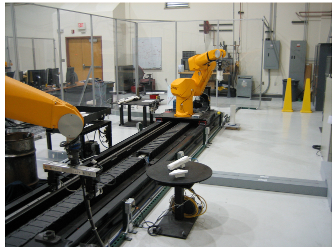
(b) Robot Transport Unit and two Staübli RX-130s.
