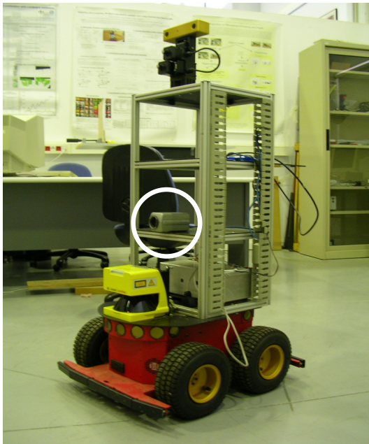
Fig. 3. Pioneer 3AT mobile platform used in the experiments
