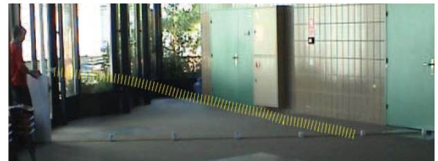
Fig. 9. Flight trajectory, launching velocity 2m/sec and launching angle \gamma = 3.5^\circ .
