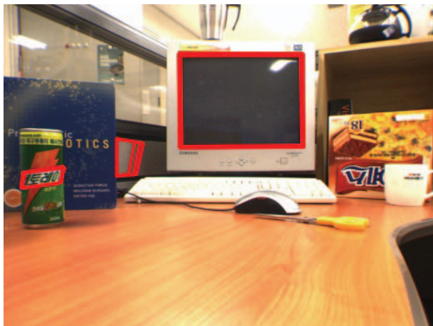
Fig. 4 The squares extracted from a scene for recognizing a monitor
