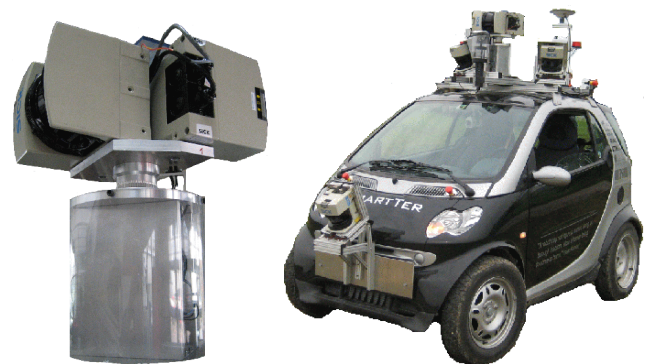
Fig. 1. The left image depicts the vertically mounted SICK LMS laser range finders which are rotated with constant speed by an electric step motor mounted under the lasers. The right image shows our robot. The robot is a standard Smart car. The model is a Smart fortwo coupé passion of the year 2005, which is equipped with a 45 kW engine.
