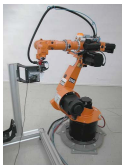
Fig. 3. "IR364" Kuka Robot Structure
