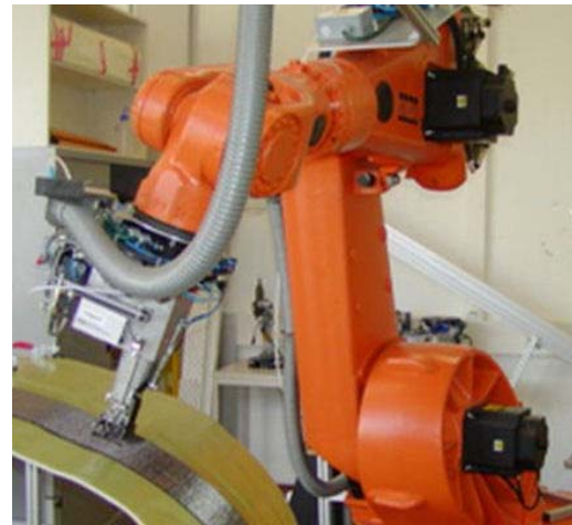
Fig. 1. Industrial sewing robot with blindstitching head.
