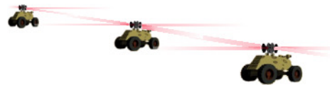
Fig. 1. The role envisioned for the UGVs. Their four motion detection sensors can pivot around a vertical axis, so that the sensors can point independently of the vehicle's orientation. When appropriately configured, they can create a "virtual fence," capable of detection of motion to and from an area of interest.
