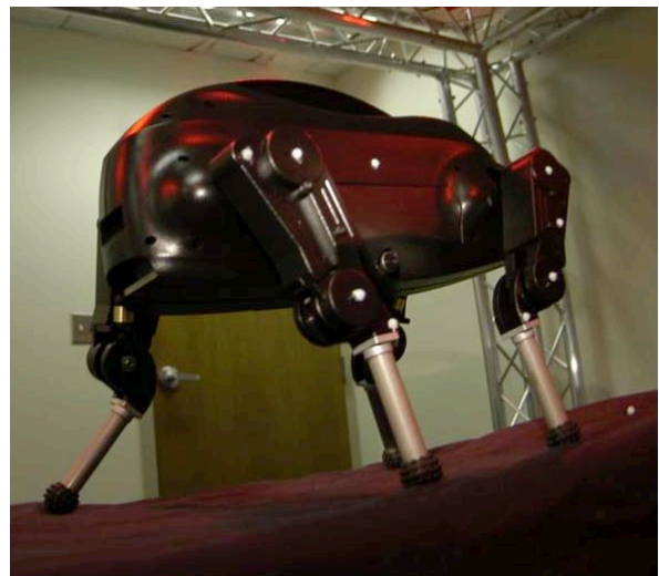
Figure 1: Little-Dog, a 3kg heavy, 40 cm long quadruped robot with 12 DOFs, produced by Boston Dynamics Incorporation.
