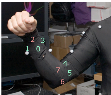
Fig. 4. Figure showing the placement of the 8 tactile actuators used in experiments. Red indicates obstructed view of the actuators.
