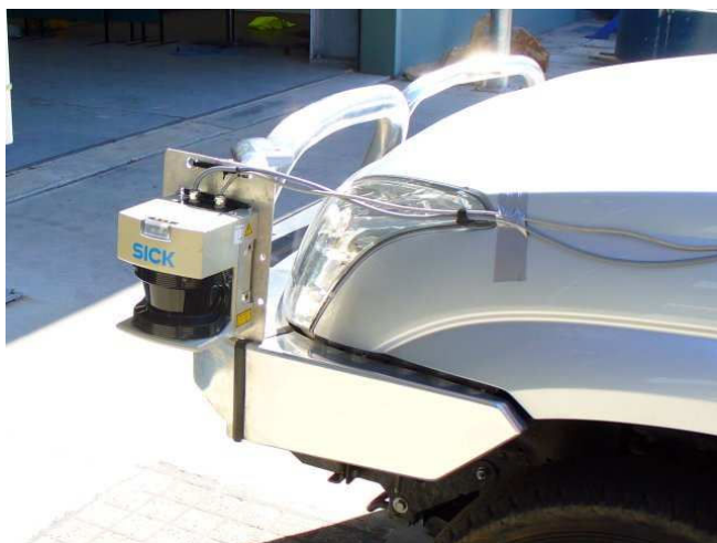
Fig. 6. The laser is mounted sideways to the front of the vehicle.
