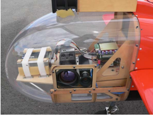
Fig. 3. Vehicle close up. An large infra-red camera (not used in this work) is visible on the left hand side. The smaller camera on the right is the visual spectrum camera used in this work. A processing stack is visible on the far right and a hard drive for logging is visible on the far left.
