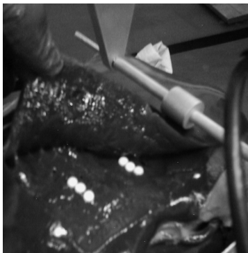
Fig. 2. Healthy liver sample with two sets of three pins spaced 26mm apart at depths of 12mm and 8mm respectively. At these depths neither pins were detectable by visual means. The wheel (15mm diameter x 15mm width) can also be clearly seen.
