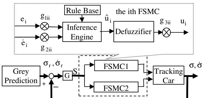
Fig. 4. Block diagram of FDSMGPC for the tracking car.
