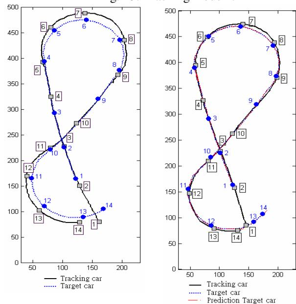
Fig. 14. Experimental result of target tracking. (a) without using grey prediction. (b) using grey prediction.
