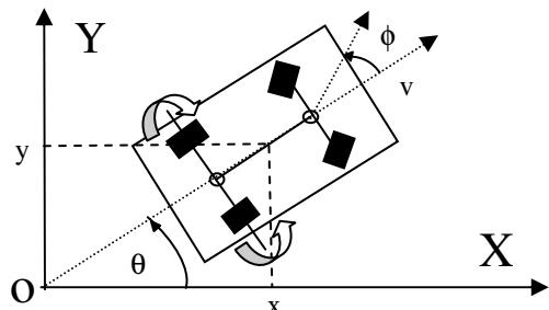
Fig. 2. Kinematic model of a tracking car.
