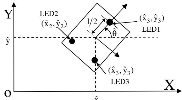
Fig. 6. The pose estimation of the tracking and target cars.
