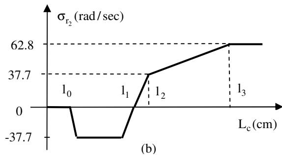
Fig. 10. The reference steering angle for the front-wheel and the reference velocity for the rear-wheel of tracking mode 1.
