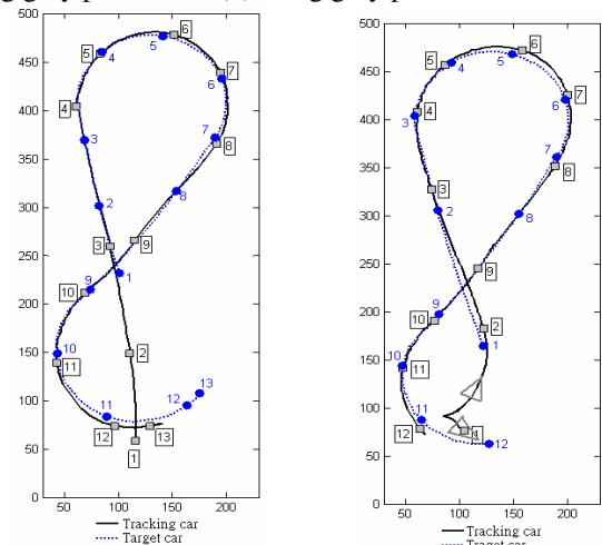
Fig. 15. (a) two seconds delay of tracking car for Figure 14(b) case, (b) different initial pose of tracking car for Figure 14(b) case.
