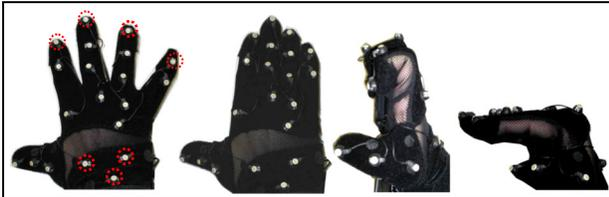
Figure 4. The calibration postures used are shown. The finger tip sensor positions marked with dashed circles are used as data points for calibration (only the first posture is marked).
