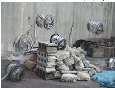
Fig. 1. Performance of Leg-in-Rotor-V: roll and jump on debris and jump again after recovering its posture
