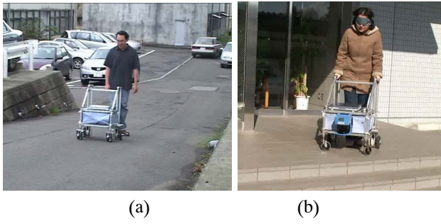
Fig. 1. Illustration of environment feedback using passive walking support system “RT-Walker” [2]. (a) Gravity compensation control (b) Stair steps detection and avoidance.
