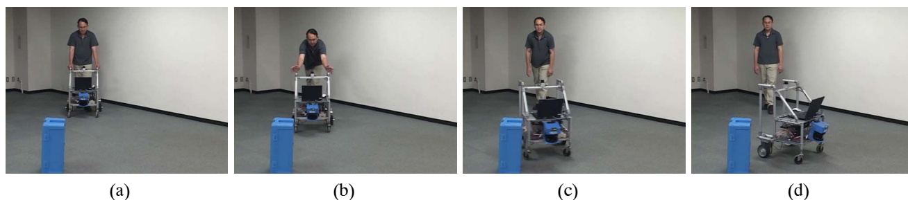
Fig. 6. Environment feedback concept for passive support system. The environment element information changes the heading angle of the support system
