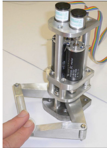
Fig.2. Interface to teleoperate and provide haptic feedback in micromotion.
