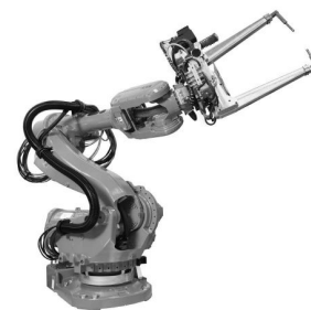
Fig. 1. IRB6600 from ABB equipped with a spotwelding gun.
