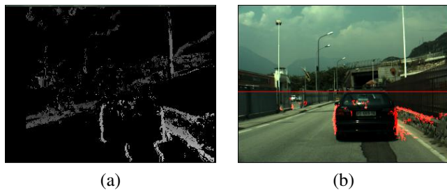
Fig. 16. Disparity image (a) detected obstacles, red pixels belong to obstacles, horizontal red line represents detected horizon(b)
