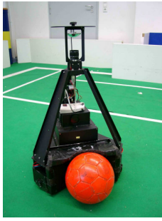
Fig. 10. The real omnidirectional robot and ball
