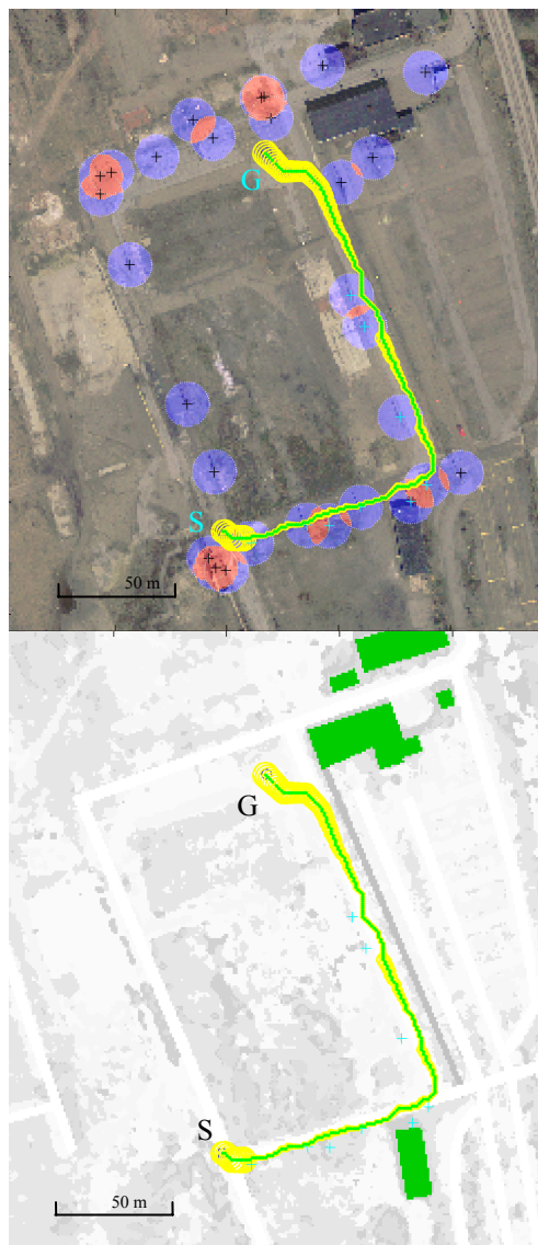
Fig 9. Path planned assuming initial uncertainty \sigma=2.5 m, uncertainty rate of 5% of distance traveled and maximum uncertainty of 10 m. The expected cost of the path is 3232, and the final uncertainty is \sigma=2.7 m. Top: aerial image and unique detection regions. Bottom: cost map used.
