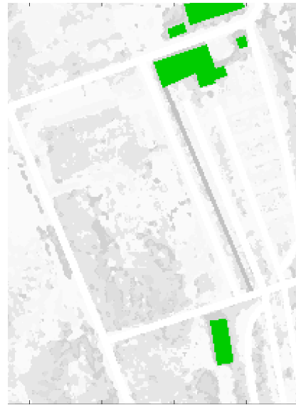
Fig 1. Cost map: lighter regions represent lower cost, and darker regions represent higher cost. Green areas are manually labeled buildings.
