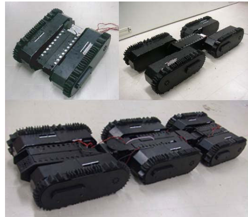
Fig. 1. Pictures of KOHGA2 that can be rearranged
