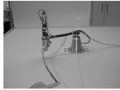
Fig. 3. Experimental 2 joint planar rigid-flexible robot manipulator
