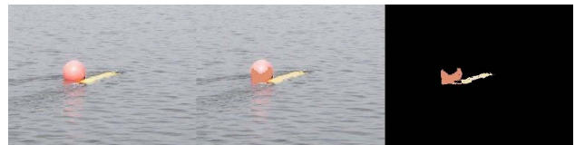
Figure 7. Image captured at test site with buoy and ISURUS AUV on surface. On top real image, real time segmented image (red, yellow) on middle and bottom (only segmented colours).
