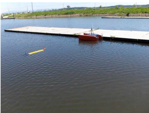
Figure 1. Roaz autonomus surface vehicle.
