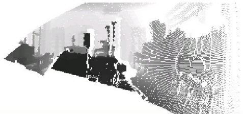
Fig. 10. Optimal projection of the second scan into the reference coordinate system.
