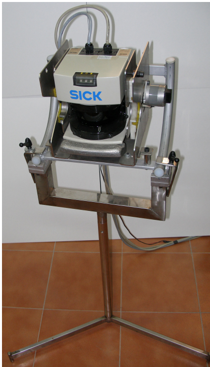
Fig. 3. The 3D laser scanner is based on a 2D rangefinder.
