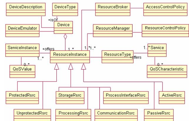
Fig. 2. Part of the proposed device model expressed in UML notation.
