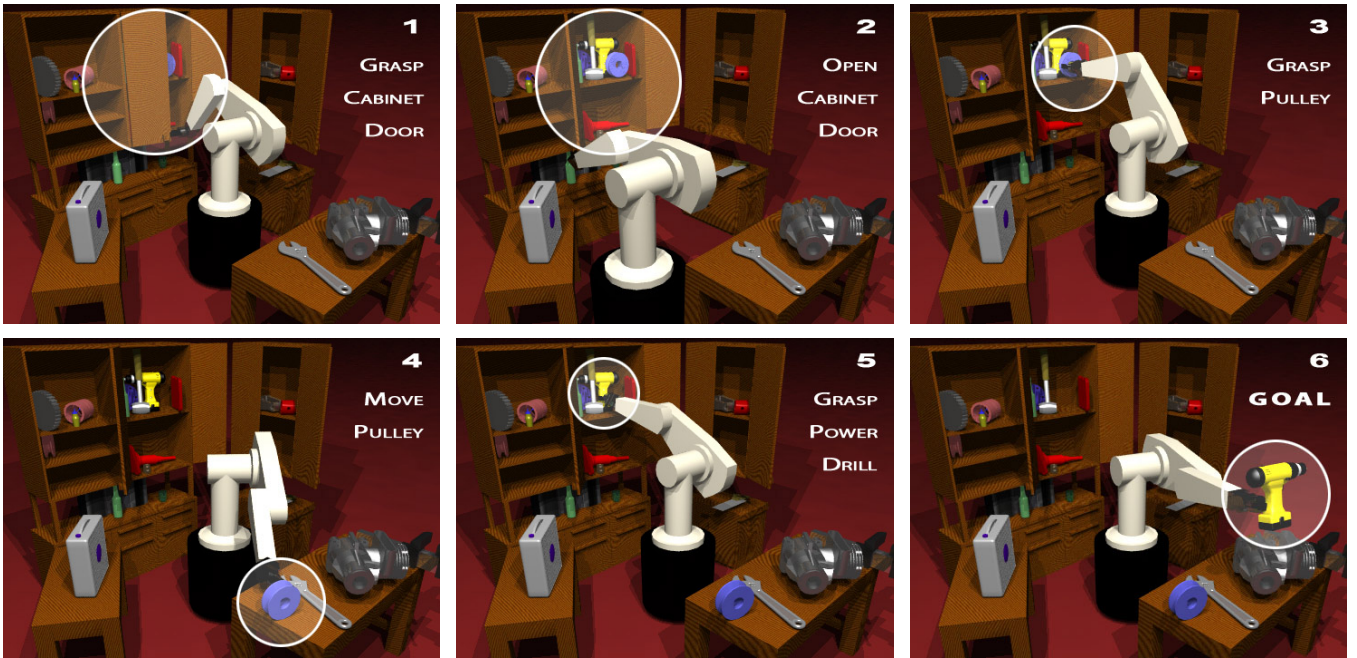
Fig. 6. Still frames from our simulation environment. In this experiment an 8-DOF mobile manipulator operates the workshop. The robot is asked to deliver the drill. RSC autonomously identifies the door and the pulley as blocking objects and generates motion plans to remove them.
