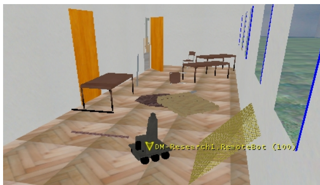
Fig. 2. In spectator mode a disembodied observer can move within the simulator without interacting with the robots, thus allowing a close observation of the performance from different points of view.
