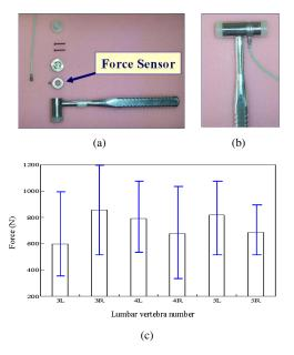
Fig. 3. Data Acquisition Experiment: (a) Parts of shock data acquisition system (b) Complete unit of shock data acquisition system (c) Force signal during hammering(L: left, R: right).
