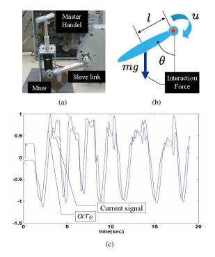
Fig. 11. Current monitoring method: (a) Experimental setup (b) Simplification of experimental setup. (c) Current monitoring Signal and calculated torque(scaled).
