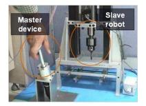
Fig. 4. 1-DOF drilling bilateral operation system.
