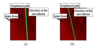
Fig. 14. Displayed images of a preplanned operation path and the direction of the end effector (the operator controls the direction of the end effector (green line) to match it to the preplanned path (black line) displayed on the spine bone image) : (a) Before operation (b) After operation.
