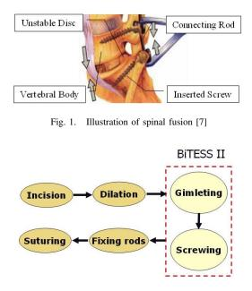
Fig. 2. Steps of spinal fusion and the roles that BiTESS II is in charge of.
