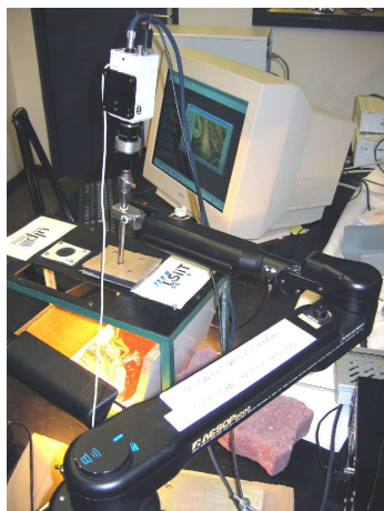
Fig. 6. The laparoscope-holder AESOP robot and the training box used for experiments with the model-free visual servoing.
