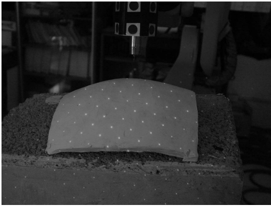
Fig. 4. Structured lighting in the form of a matrix array of laser spots.
